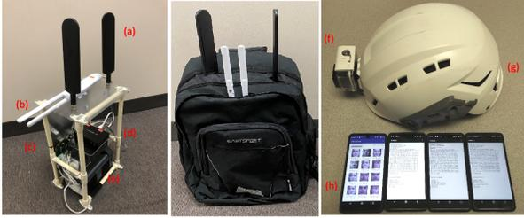
Fig. 3: DistressNet-NG hardware components: a) LTE antenna, b) Wi-Fi AP, c) LTE eNB, d) Intel NUC with LTE EPC and HPC; e) Battery; f-g) Helmet with body camera; h) Mobile devices
