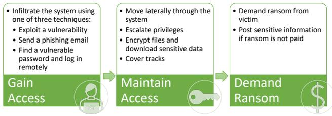
Figure 3: Ransomware attack phases that Babuk typically uses on their victims, including the DCMPD [22].
