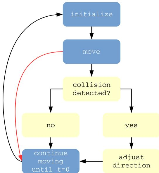
**Figure 4: Simplified block diagram of collision avoidance.**
