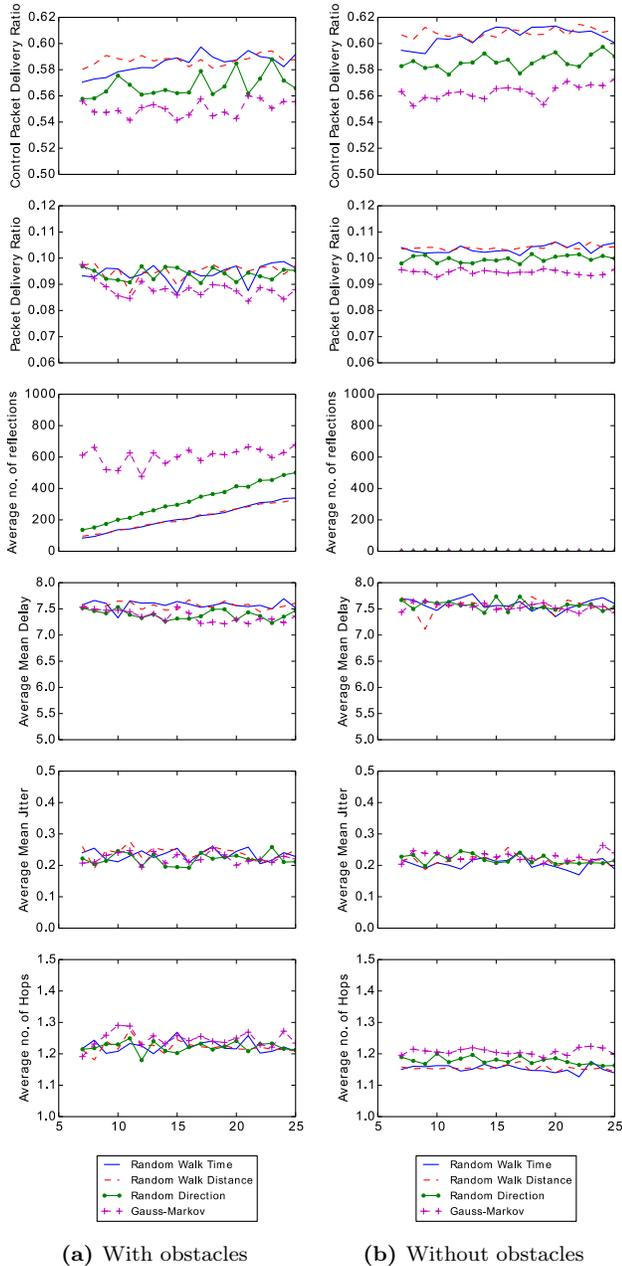
Figure 7: Network performance parameters.
