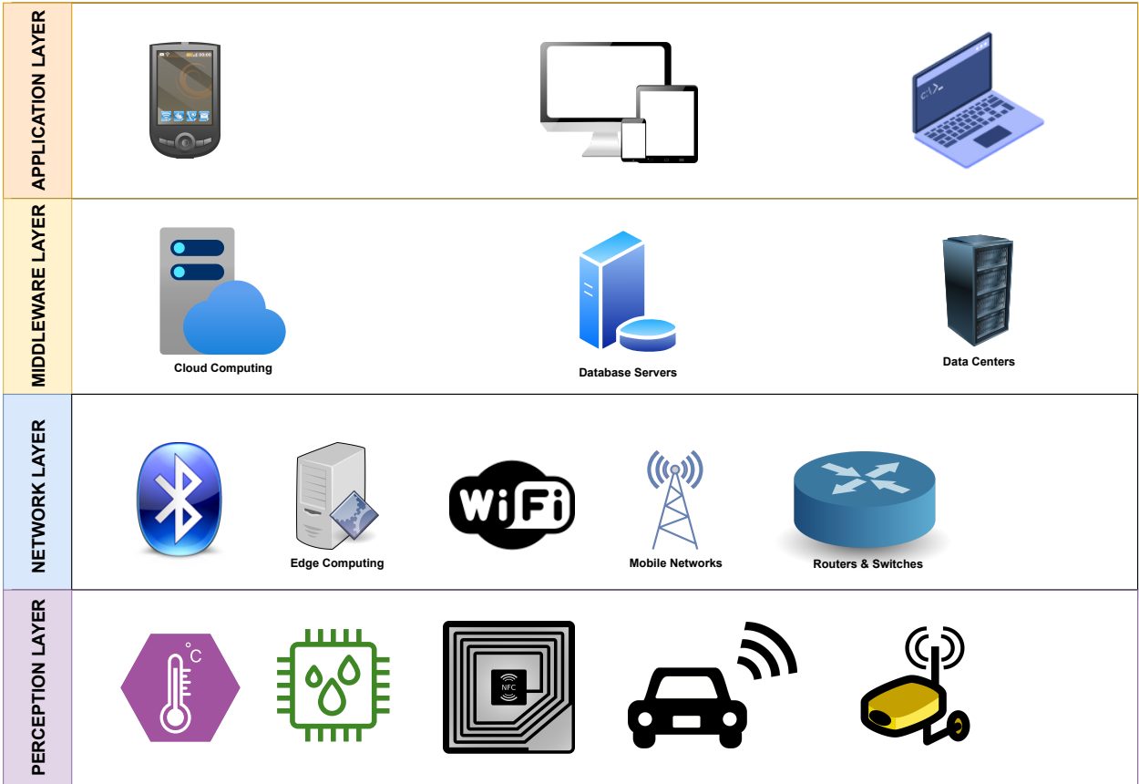
Figure 2.2: The 4 Layer IoT Architecture
