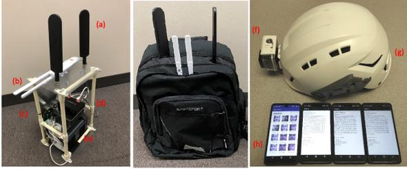
Fig. 3: DistressNet-NG hardware components: a) LTE antenna, b) Wi-Fi AP, c) LTE eNB, d) Intel NUC with LTE EPC and HPC; e) Battery; f-g) Helmet with body camera; h) Mobile devices
