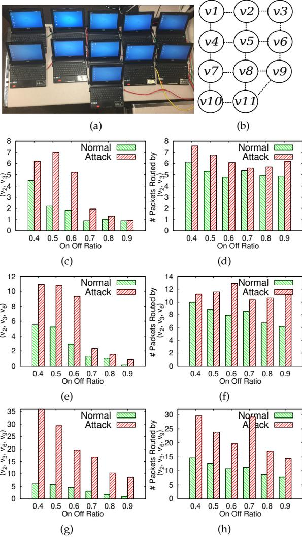
Fig. 2: (a) Attack implementation testbed. (b) Network topology. Routed packets for HRP (c, e, g) and Prophet (d, f, h).
